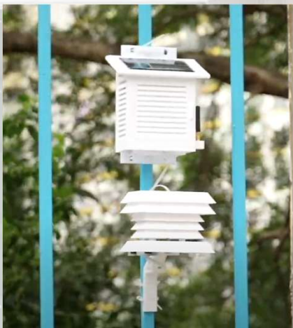
Citizen Science weather station (Arduino-based 3D print)
