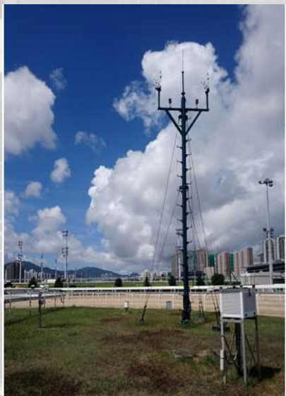
Conventional weather station (AWS – Automatic Weather Station)
